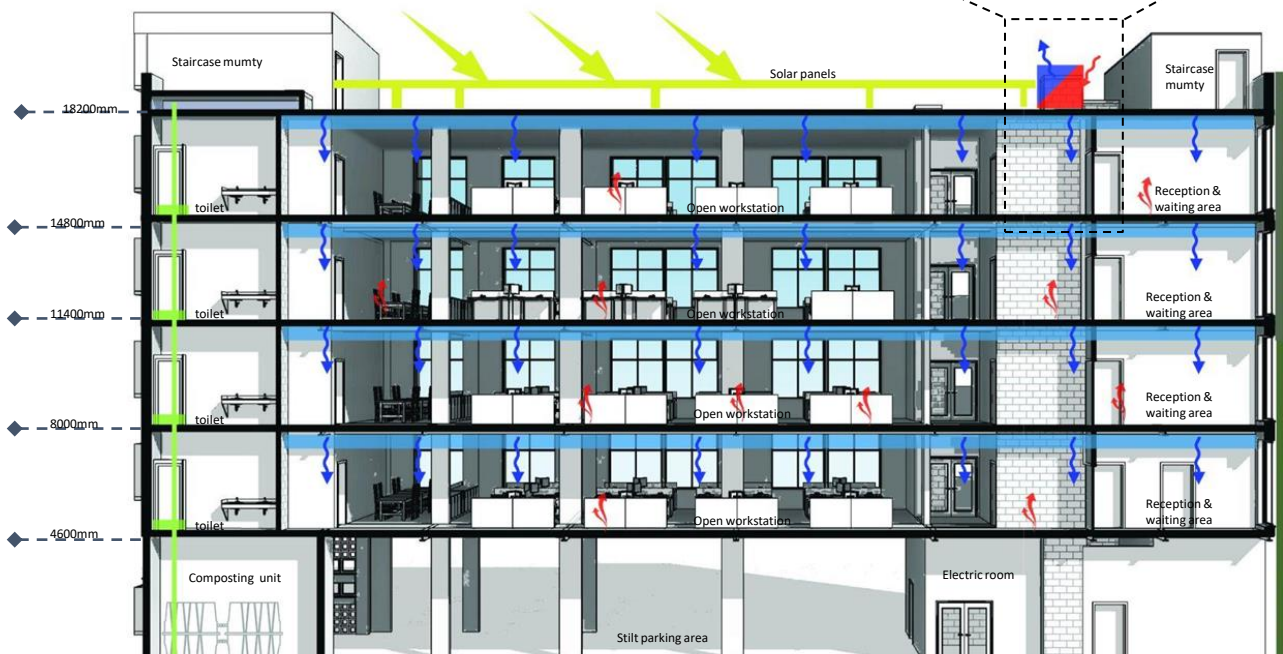
Fig 49: Operational Zones for Air-conditioning for typical office floor
